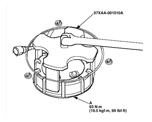
8. Remove the locknut (A) and the fuel pump/sender assembly.
